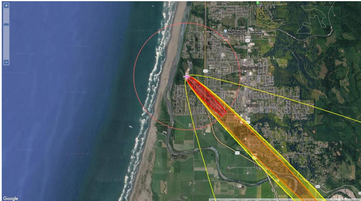
Figure 4. ALOHA Worst-Case Scenario Threat Zones Map and Circle of Concern Chlorine Release 1.0miles.
