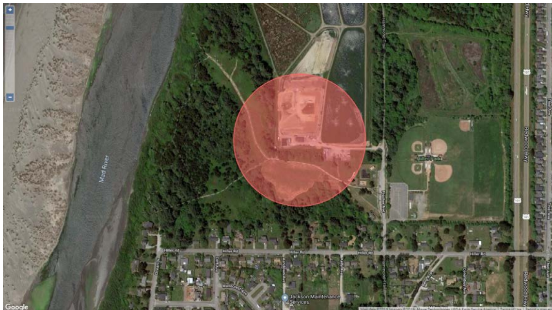
Figure 2. RMP*Comp and ALOHA Alternate-Case Scenario Circle of Concern for both Chlorine and Sulfur Dioxide. <0.1miles
