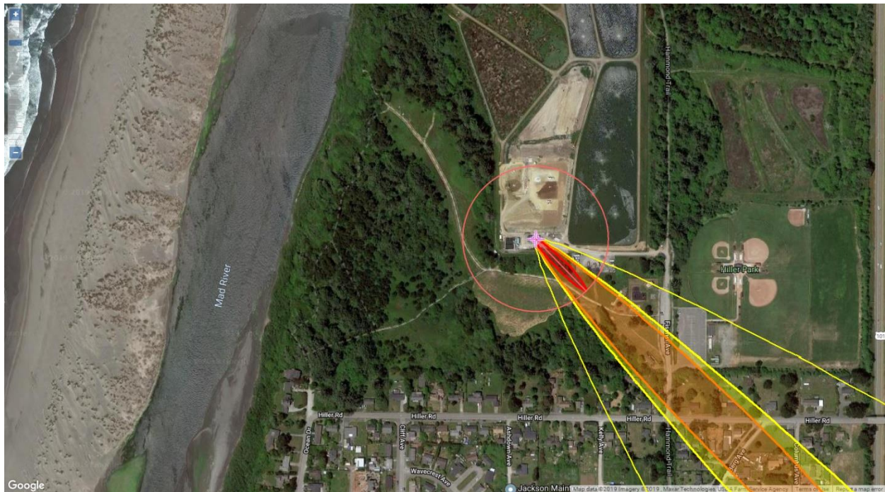
Figure 12. ALOHA Alternate-Case Scenario Threat Zones Map and Circle of Concern Sulfur Dioxide Release <0.1miles.
